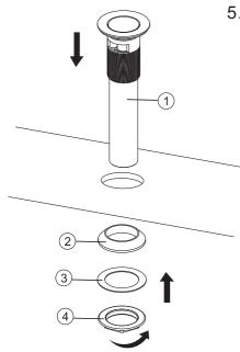
5. From the top of the drain hole, place the drain ① through the installation hole. From under the drain hole, install the thick washer ②, washer ③ and nut ④ by hand twisting on to the tail pipe of the drain. Then, install the tail pipe to the wall plumbing. Use of plumbers putty or silicone is recommended to seal drain ① to top side of bowl.
