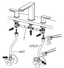
4. Connect the water supply lines to the bottom ends of the "quick connect" hose (#7) and to the hot and cold water supply valves. Secure and tighten with an adjustable wrench.
