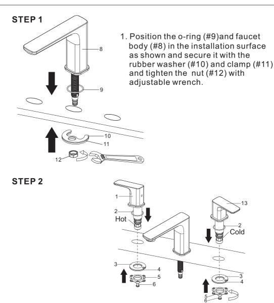
2.Position the o-ring (#2) and handle mounting (#1,#13) in installation surface as shown and secure it with kit (#3,#4,#5,#6) and tighten the screws with screwdriver. Repeat the above steps for the other handle.
