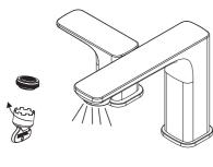
6. Remove the aerator with an aerator wrench (a quarter or flat surface tool could also work). Turn the faucet handle all the way on, turn on the hot and cold water supply and flush water lines for one minute. Reinstall the aerator with an aerator wrench.
